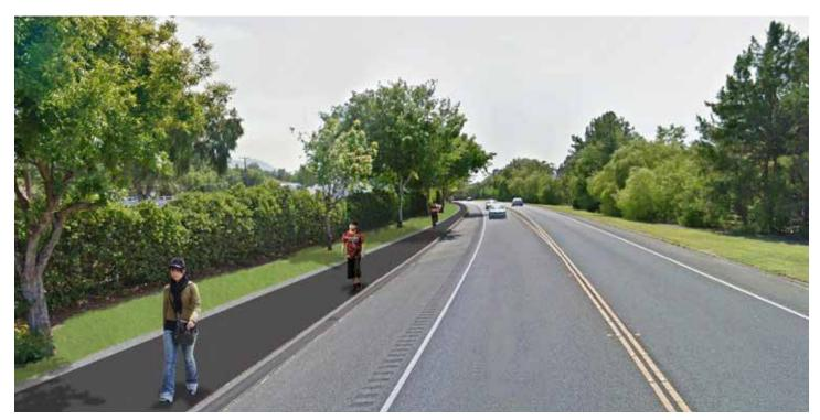
**CONCEPTUAL DESIGN ONLY:** Narrowing the street by adding a sidewalk slows down vehicles and has the added benefit of providing another transportation mode option for students.
