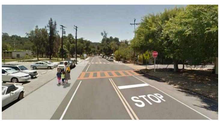
**CONCEPTUAL DESIGN ONLY:** Installing of a stop sign and advance yield line indicates vehicles need to stop and look for pedestrians or other vehicles. Installing a second high visibility crosswalk allows pedestrians to cross away from a conflict point.
