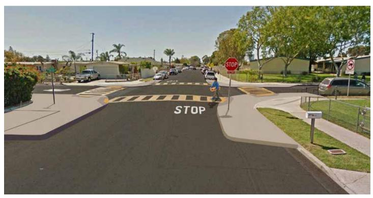
**CONCEPTUAL DESIGN ONLY:** Installing a stop sign indicates vehicles need to stop and look for pedestrians or other vehicles. Installing a curb extension slows down vehicles and has the added benefit of indicating where pedestrians should cross.
