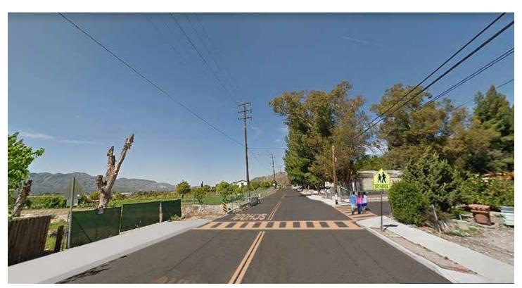
**CONCEPTUAL DESIGN ONLY:** Filling a sidewalk gap and adding a high visibility crosswalk complete the connection to school.
