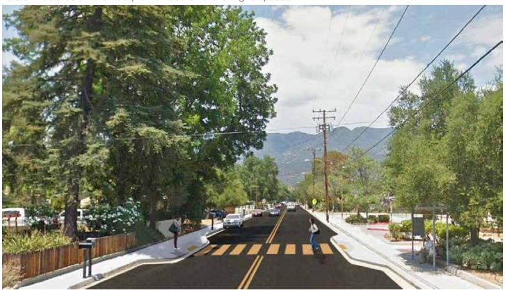
**CONCEPTUAL DESIGN ONLY:** Installing curb extensions along with a high visibility crosswalks slows down vehicles and has the added benefit of indicating where pedestrians should cross and shortening the distance they have to cross.
