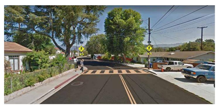
**CONCEPTUAL DESIGN ONLY:** Installing a high visibility crosswalk along with Rectangular Rapid Flashing Beacons indicates where pedestrians should cross along with alerting vehicles to yield to pedestrians.
