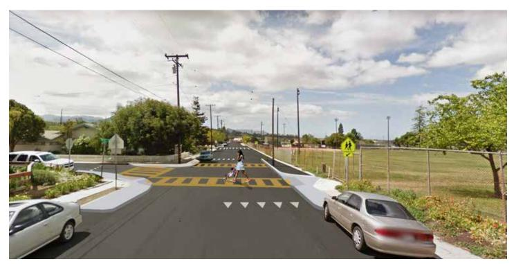
**CONCEPTUAL DESIGN ONLY:** Installing advance yield teeth indicates vehicles need to yield and look for pedestrians or other vehicles. Installing a curb extension along with a high visibility crosswalks slows down vehicles.
